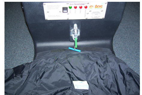
Octi-Dry Secured to E-TES Snout
